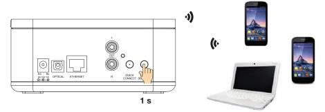
The LED indicator is flashing few ties then light then becomes permanent wnite: the unit becomes detectable as a WiFi access point.
