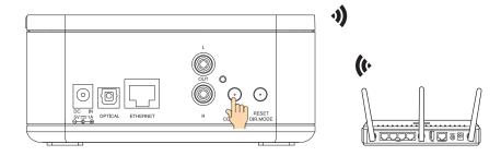
Press the WPS key of the router and the Quick Connect key of the playconnect simultaneously. The LED is flashing fast (white). After around 10~ 40 seconds, the WiFi LED on the device becomes permanent white: The unit is connected to your network.
