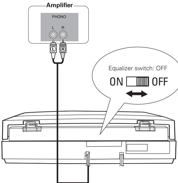
When connecting to an AUX input terminal or an input terminal other than "PHONO"
