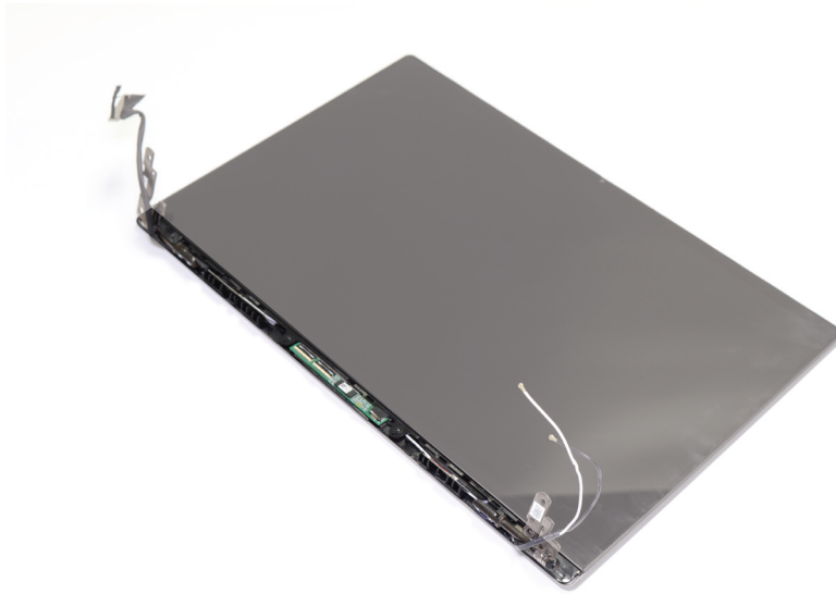
Figure 32. Assemble the EDP cable, glass rubber frame, and antenna cable
