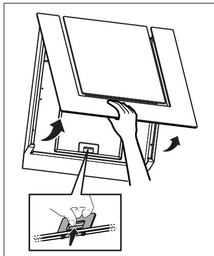
**4.2 NON-washable activated charcoal filter** - The saturation of the **charcoal filter** occurs after more or less prolonged use, depending on the type of cooking and the regularity of cleaning of the grease filter. In any case it is necessary to replace the cartridge at least every four months. The charcoal filter may NOT be washed or regenerated.
