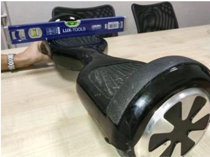
After making sure that both wheels are properly levelled, press POWER button and hold it for 5 seconds until blue diodes start to flash.
